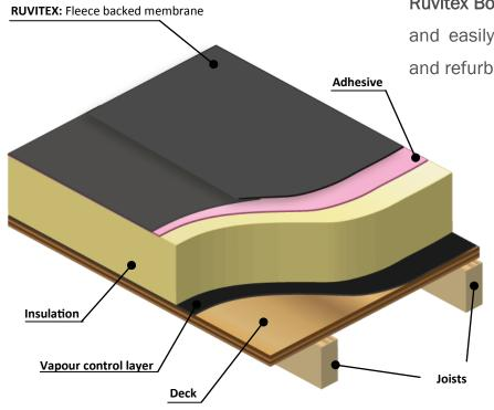
Ruvitex Bonded System is a flame free, clean and easily installed roofing system for new and refurbishment projects.
