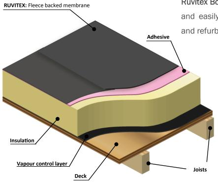
Ruvitex Bonded System is a flame free, clean and easily installed roofing system for new and refurbishment projects.
