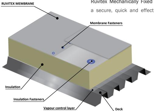
Ruvitex Mechanically Fixed Overlap System provides a secure, quick and effective solution on new and
